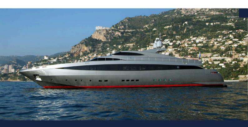
The other unit designed by Tommaso Spadolini and delivered in 2005 is Nina J. Slightly longer than the RC, 42.20 metres, it uses a similar line, with a reverse sheerline, still completely wide body, but less accentuated. The color is a discreet silver gray and has a pilot capsule above the superstructure of the upper deck which distinguishes it from its smaller sister. Always built in aluminum and powered by the same pair of MTU and KaMeWa wateriets, it reaches a maximum speed of 32 knots.
